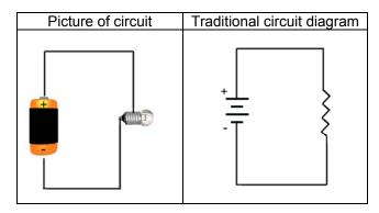
11. Make a traditional circuit diagram for the circuit shown below. Use the resistance symbol (^^^) to represent the light bulb in the circuit. Be sure to correctly label the terminals of your battery.
