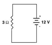
5. Calculate the current for the circuit shown to the right. Be sure to use appropriate units.
