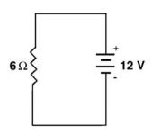
6. Calculate the current for the circuit shown to the right. Be sure to use appropriate units.
