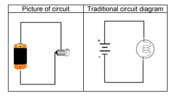
The traditional representation of voltage sources, such as batteries, is an alternating series of long and short lines
